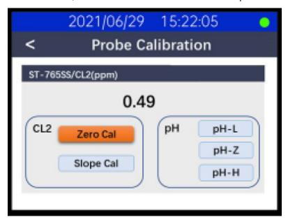
**Zero Calibration.** Select Zero Cal from the Probe Calibration screen. Put the probe into the Zero standard solution. After the probe is stable for at least 10 minutes, click the Enter button to start calibration.
