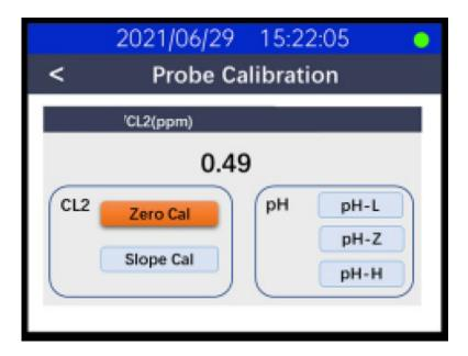
PH-L calibration. Remove and place the FCL700 probe in the pH 4.0 standard solution, measure for 1 minute and wait for the measurement result to stabilize. Click the Enter button to start the PH-L calibration.
