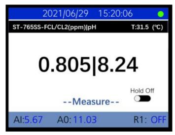
Long press OK button for 3 seconds on the main interface to open the HOLD - ON/ OFF page. The cursor shows black is the selection mode, and blue is the editing mode. Click the OK key to enter the editing mode, and the up/down keys can be used to adjust the value of the setting item. Once set where desired, click the OK button to start the HOLD-ON function.
