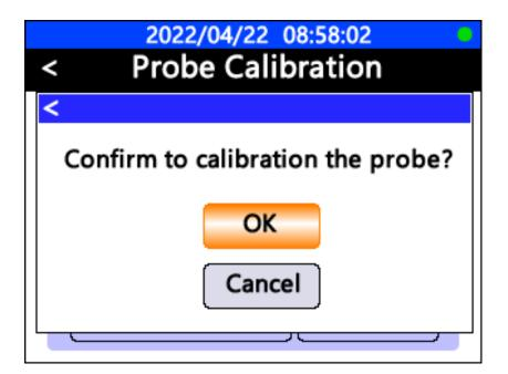
PH-Z (mid) calibration. Remove and place the FCL700 probe in the pH 7.0 standard solution, measure for 1 minute and wait for the measurement result to stabilize. Click the Enter button to start the PH-Z calibration.
