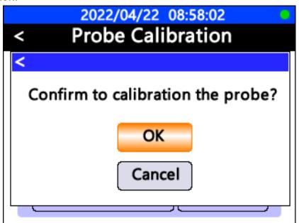
Select the Enter button on the probe confirmation page. The controller will them perform a calibration for the probe, and will wait for the calibration result. The probe calibration result will be automatically displayed on the calibration interface.
