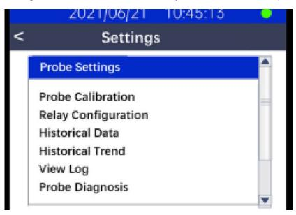
Select the probe setting to enter the desired Probe Type setting interface. The TS05 supports manual selection of the probe type or automatic identification of the probe type. Us the Up/Down arrows to select the probe type. Select FCL700.
