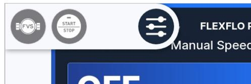
**IMPORTANT:** To begin operation, press the START button to place pump in STANDBY. The display background will turn yellow indicating the pump has been stopped remotely. When the pump is started by the remote contact, the display background will turn green.
