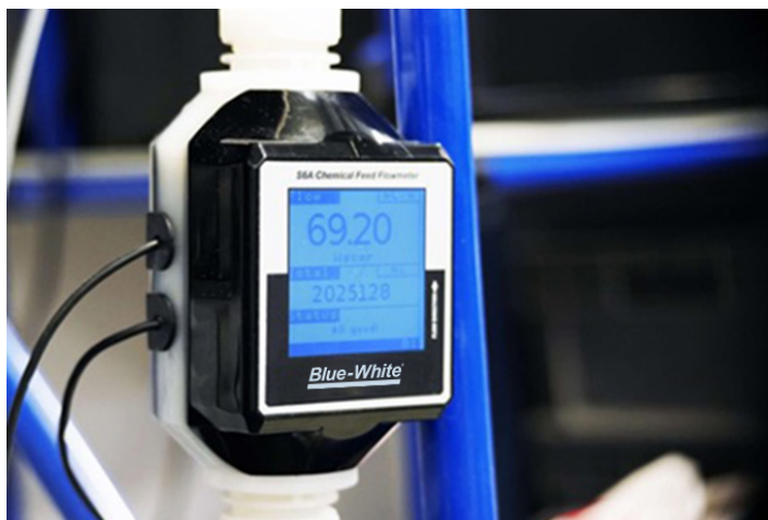
Figure 1. Blue-White's ultrasonic chemical flow meters utilize strainers to break up bubbles and reduce interference with the measurement signals. The addition of a temperature sensor and an integrated algorithm allows the unit to compensate for temperature variations that would otherwise result in inaccurate readings. Altogether, the system can accurately measure liquid chemical feed with flow rate readings as low as 10 mL/min.
