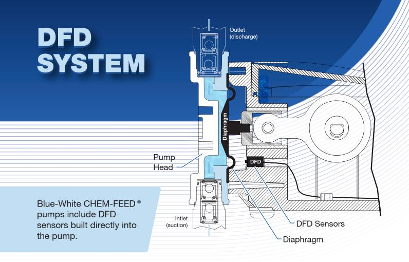
Although it doesn't happen often, diaphragm failure can occur. The DFD sensors will detect the chemical behind the diaphragm caused by diaphragm failure. The pump will then shut down and energize a relay switch. This permits communication with external equipment such as a backup pump, SCADA system, or alarm. It also serves to prevent chemical spills and added downtime.
