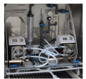
Peristaltic pumps easily prime under maximum pressure but are usually limited to maximum discharge pressures of around 125 psi. In addition, they are capable of injecting into a vacuum without the need for metal spring loaded valves. Their output
