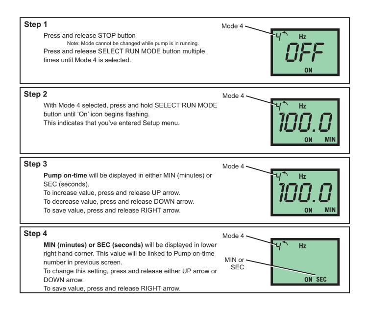
**Time-out** - Flex-Pro pumps have a time-out setting of 20 seconds while in configuration menus. If built-in timer exceeds 20 seconds without a button being pressed, then pump will exit configuration menu. Changes will only be saved after RIGHT arrow button is pressed and released.
