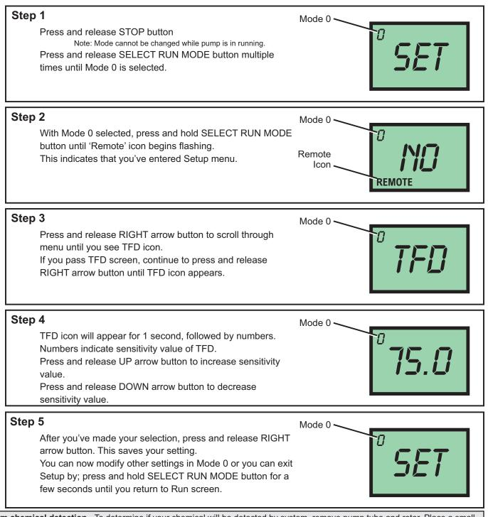
**Confirm chemical detection** - To determine if your chemical will be detected by system, remove pump tube and rotor. Place a small amount of chemical in bottom of pump head - just enough to cover sensors. Turn on pump. If TFD system detects chemical, pump will stop after two seconds and TFD alarm screen will display. Press STOP button to clear alarm.
