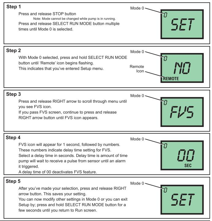
**Time-out** - Flex-Pro pumps have a time-out setting of 20 seconds while in configuration menus. If built-in timer exceeds 20 seconds without a button being pressed, then pump will exit configuration menu. Changes will only be saved after RIGHT arrow button is pressed and released.
