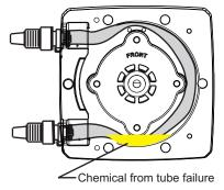
If system has detected chemical, pump tube must be replaced and pump head and roller assembly must be thoroughly cleaned. Failure to clean roller assembly will void warranty.
