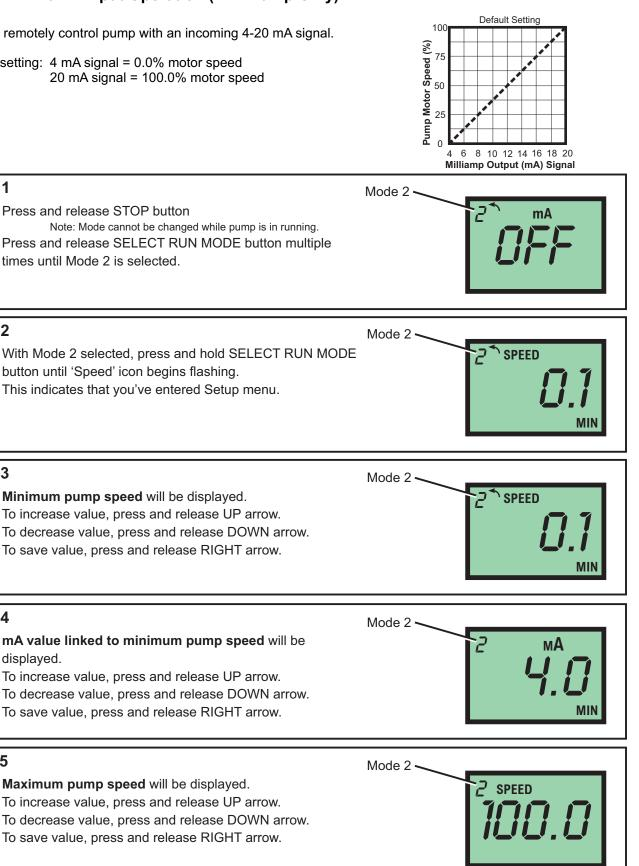
Time-out - Flex-Pro pumps have a time-out setting of 20 seconds while in configuration menus. If built-in timer exceeds 20 seconds without a button being pressed, then pump will exit configuration menu. Changes will only be saved after RIGHT arrow button is pressed and released.
