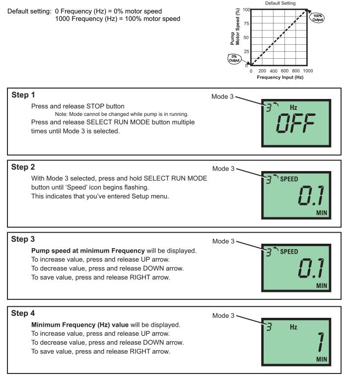
**Time-out** - Flex-Pro pumps have a time-out setting of 20 seconds while in configuration menus. If built-in timer exceeds 20 seconds without a button being pressed, then pump will exit configuration menu. Changes will only be saved after RIGHT arrow button is pressed and released.
