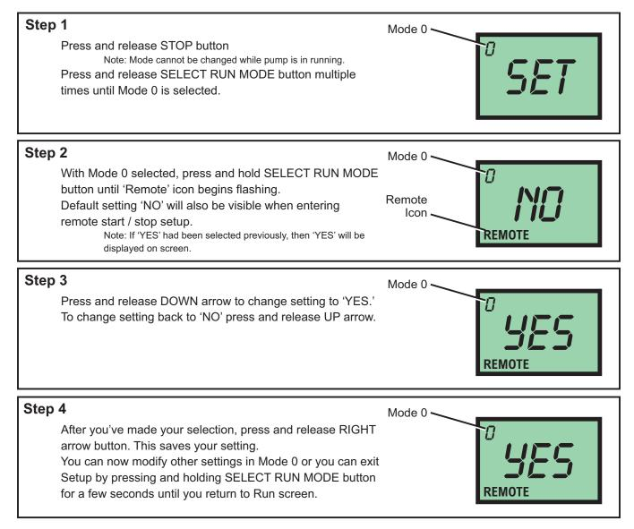
Running pump with Remote Start / Stop enabled, 'REMOTE' icon will always be visible on lower left side of screen. Pump will display 'STBY' (standby) if pump is in stop mode via contact closure signal. **Please use caution in this mode, pump can start at anytime. If you must perform maintenance to pump, press and release STOP button.**
